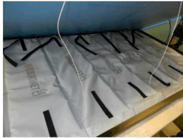
Heater blankets installed behind module
