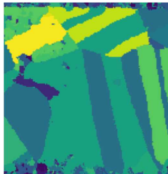
Left: example of a grain region selected Right: a convex hull is constructed from the region, and all points in the hull are assimilated
