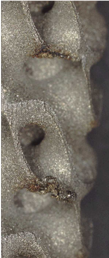
Figure 47: KEYENCE image of a printing error caused by an overhang
