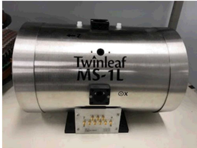
Twinleaf MS-1L shield with QuSpin Gen-2.0 QZFM inside
