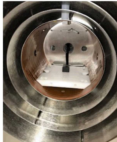
Twinleaf MS-1L shield with QuSpin Gen-2.0 QZFM inside
