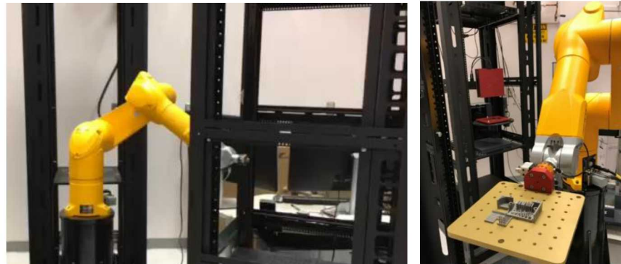
robotic work cell for material characterization
