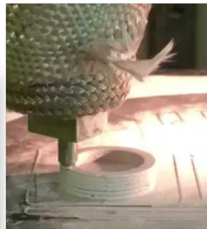
ceramic-thermoplastic 3D (CT3D) printing alumina
