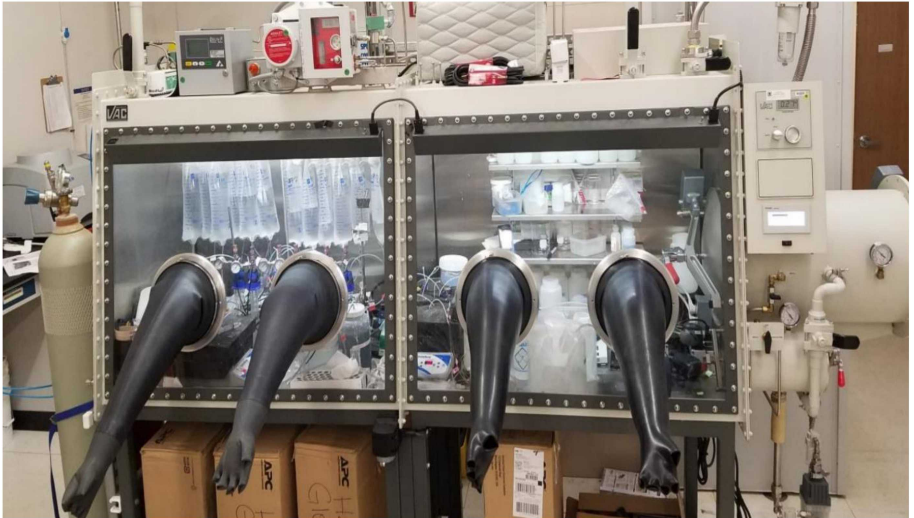
Figure 2. Glovebox setup for anaerobic flow-through experiments at Sandia Carlsbad facilities.
