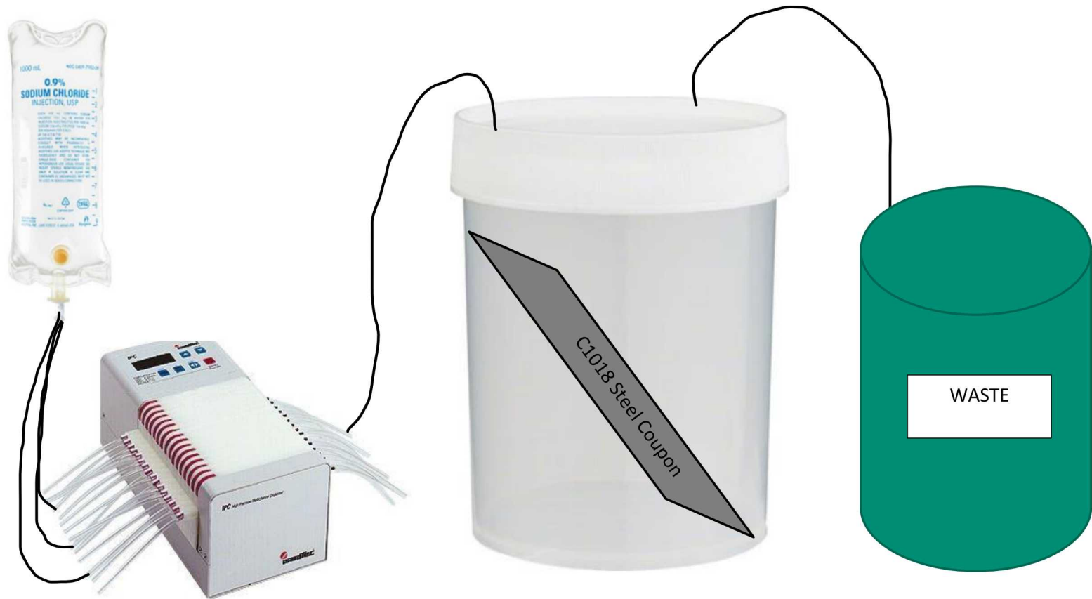
Figure 3. Simplified schematic of flow-through setup process
