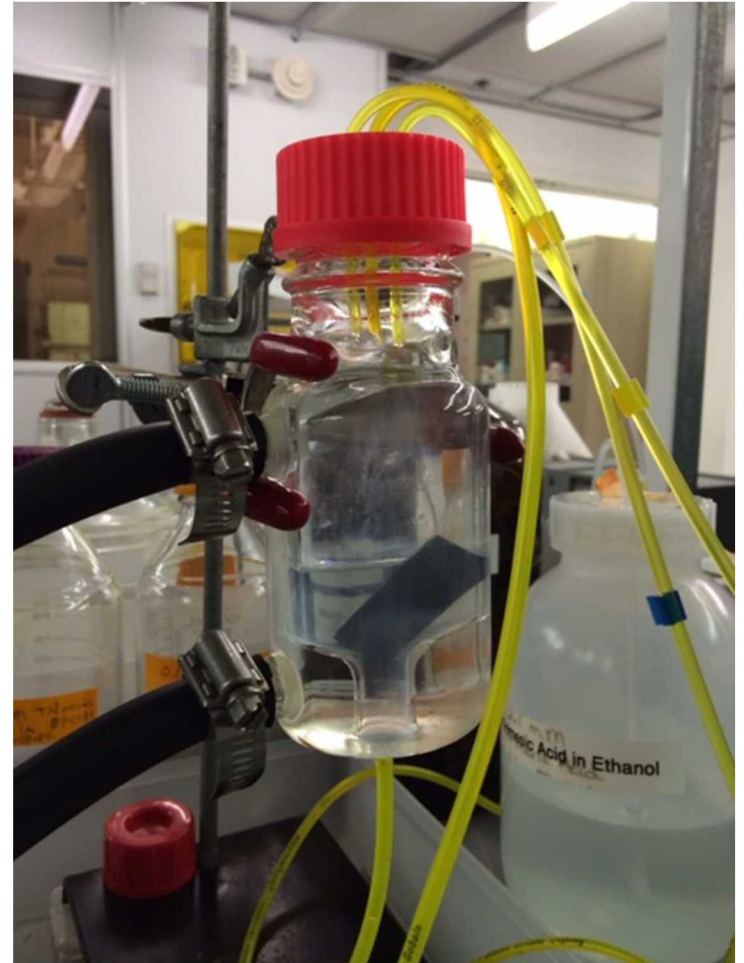
Automated MOF film growth with QCM capability
