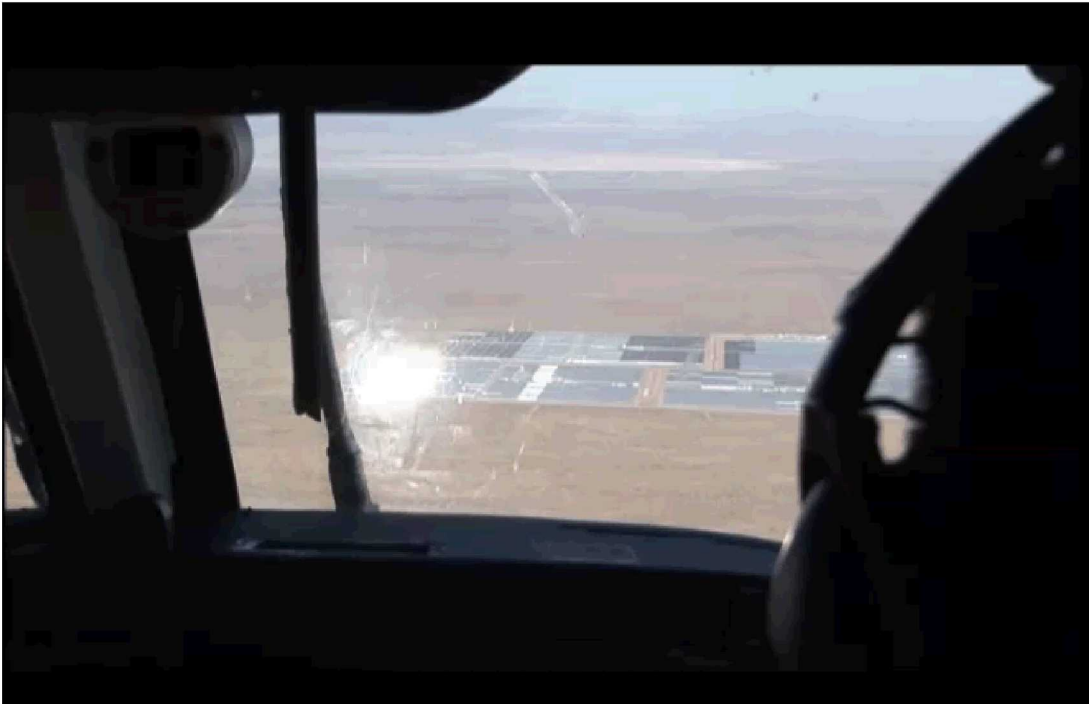
Glare observations from C-12 cockpit at Kramer Junction, CA (from Air Force Flight Test Center 412 TW at Edwards AFB, approval #13166)
