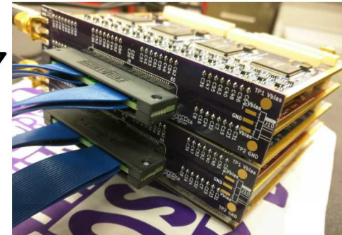
Full 64/128 channel electronics module (Custom IRS3D ASICs)
