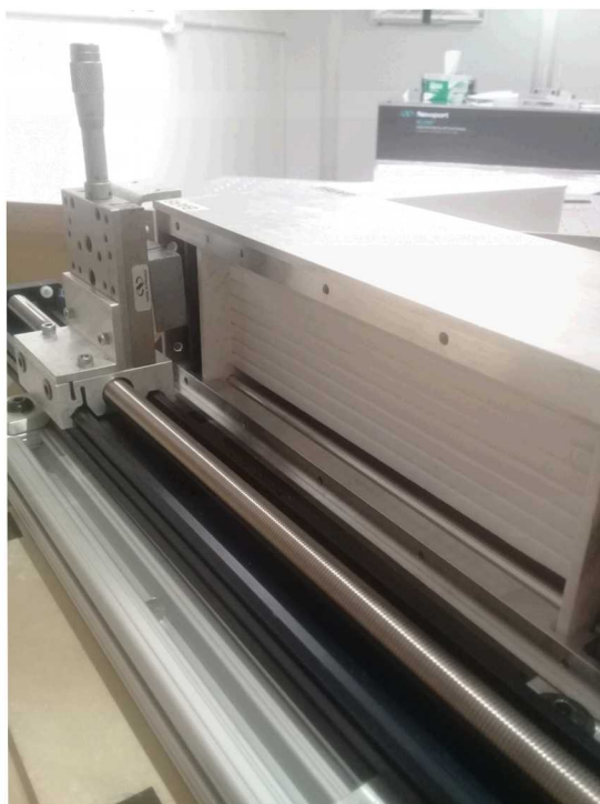
Sr-90 Source w/ Collimator Scanned Along Array
