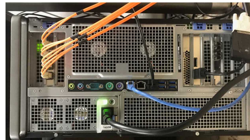
Dell 7920 16-core workstation + CAEN A3818 optical interface
