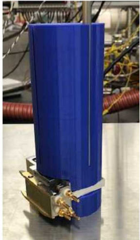
33mm MCP in Ceramic holder Inserted in ALD precursors path
