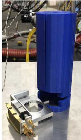
33mm MCP in Ceramic holder Inserted in ALD precursors path
