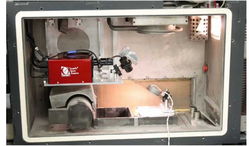
ThermaViz installed in the 3D Systems ProX 200
