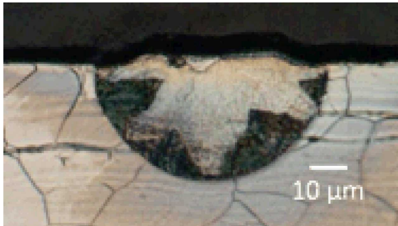
melt pool on plate, 100W, 1500 mm/s
