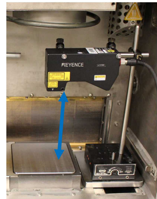
Keyence LJ-V7200 focused onto build plate
