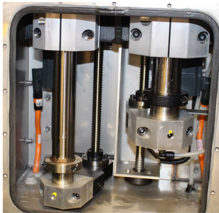
supply piston drive (left) & build piston drive (right)
