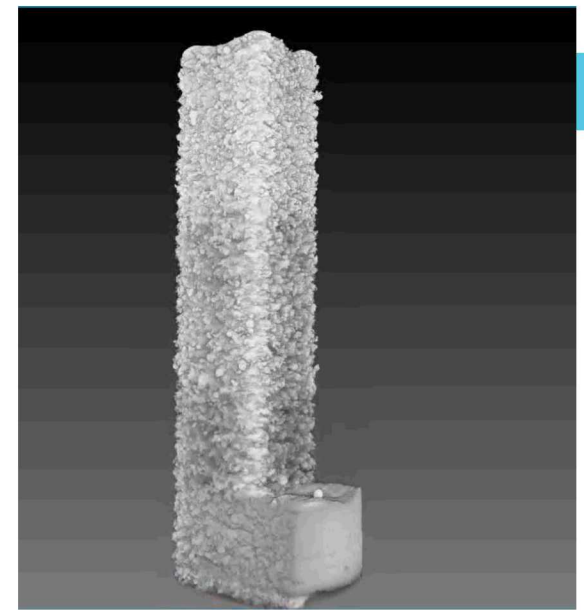
captured defect holes part CT image
