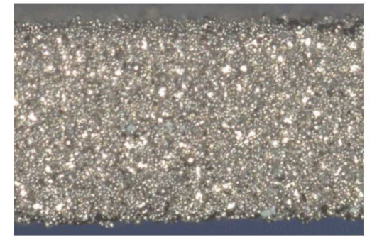
as-printed 316L SS, S_a = 26.8\mu\text{m}
