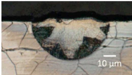
melt pool on plate, 100W, 1500 mm/s
