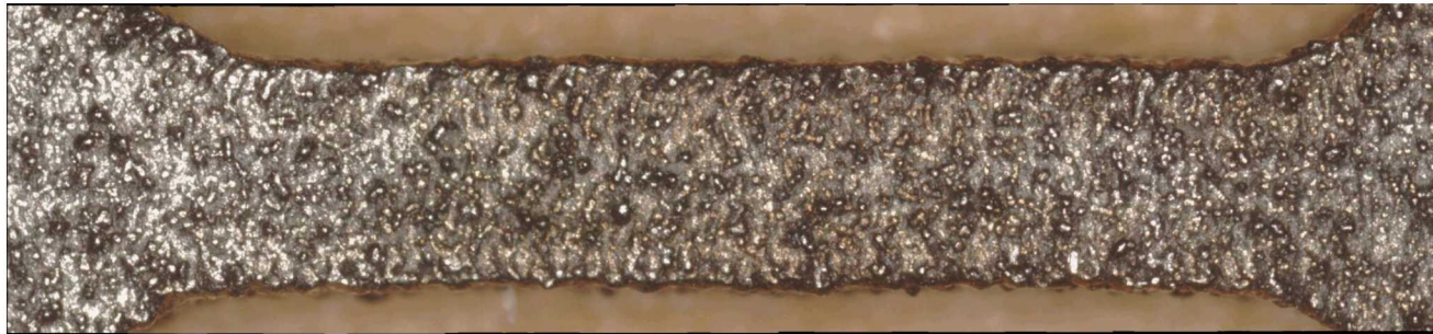
17-4PH dogbone surface roughness
