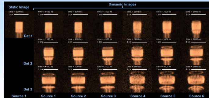
Images were phase matched over 3 detonators using six sources in each shot. Images from 7500 ns to 9000 ns display effect of image parallax, the detonator appears to rotate.
