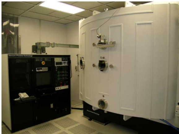
Coating system in class 100 (ISO 5) clean room
