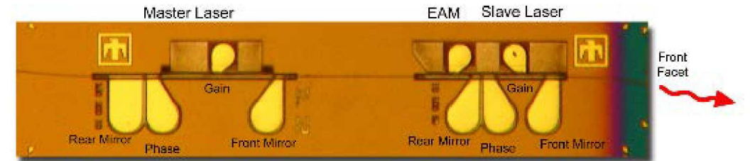
On-Chip Injection Locking Enhanced Modulation > 50 GHz, C-Band
