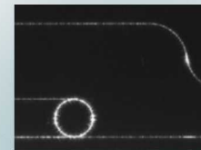
Alumina ring filter /waveguide for visible wavelength
