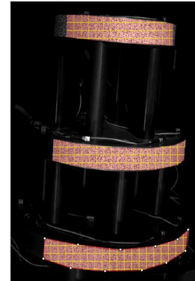
Subset 21 px, Step 10 px (352 Subsets)
