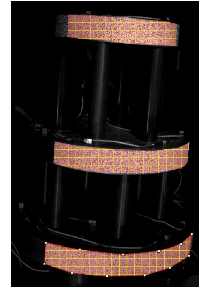
Subset 21 px, Step 10 px (352 Subsets)
