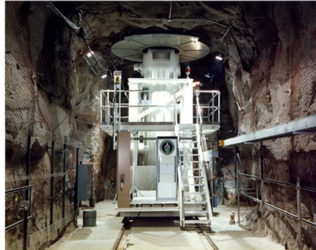
Rail-mounted canister transfer and emplacement machine, main gallery (in receive position under waste handling borehole)
