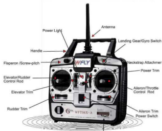
WFT06X-A Transmitter Features (Front)
