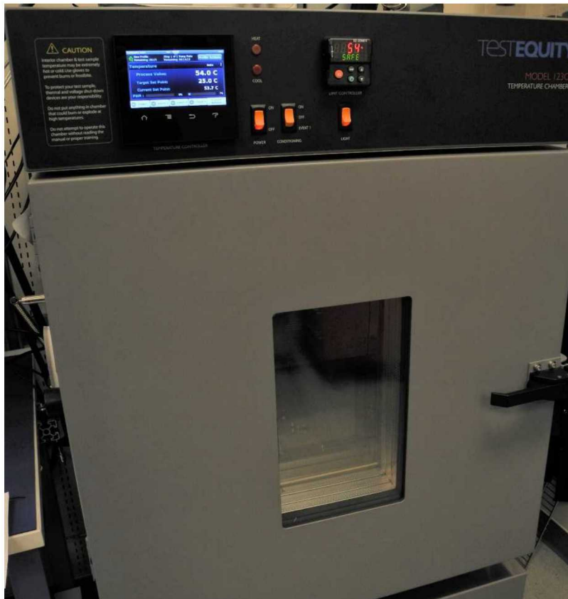
Fig. 9. Temperature chambers used for thermal cycling
