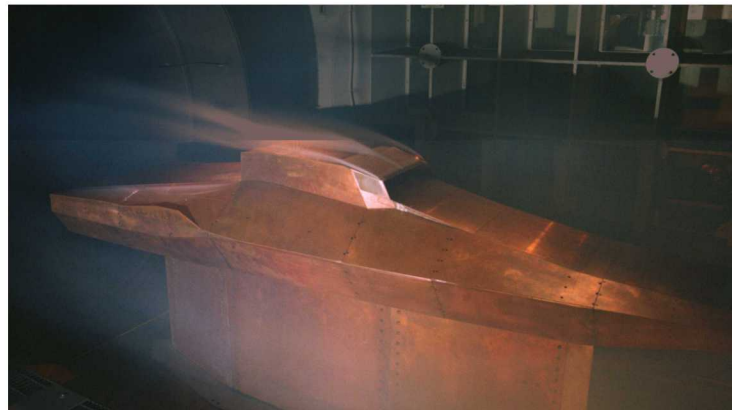
NASA X-43A experimental unmanned hypersonic vehicle (left) CFD simulation of Mach 7 flight (right) Mach 7 wind tunnel test full-scale X-43A. Images courtesy of www.dfrc.nasa.gov/Gallery/Photo/X-43A/Large/
