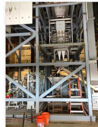
Solex/VPE/Sandia particle/sCO 2 shell-and-plate heat exchanger
