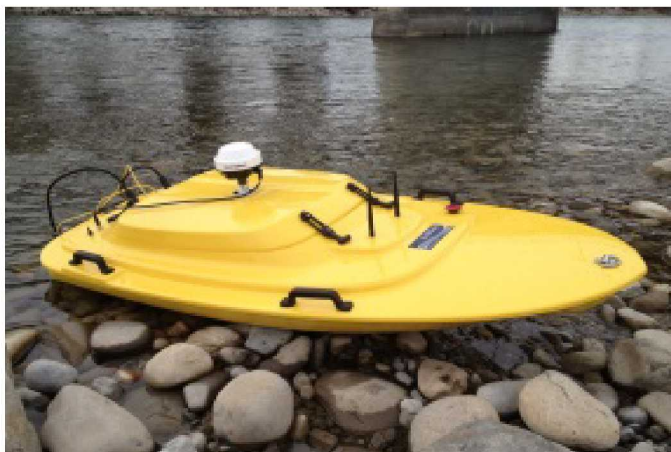
Remote control boat with RTK GPS
