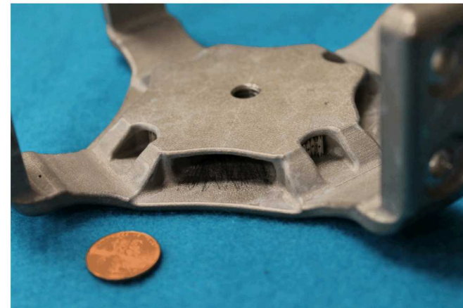
final part after polishing, machining & manual support removal
