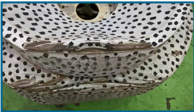
Two Used Impact Limiters from 2010 Tests (bottom one is shown)
