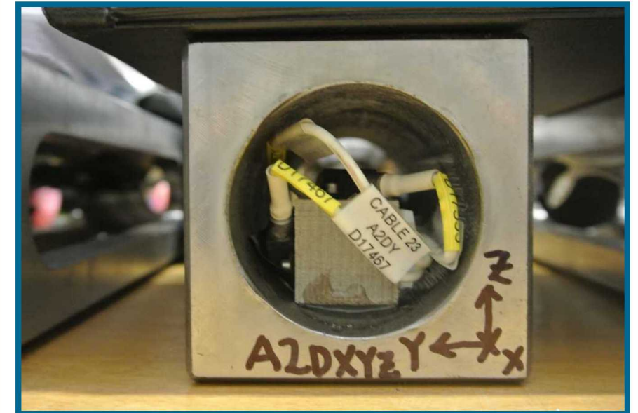
Tri-Axial Accelerometer Block A2DX, A2DY, and A2DZ
