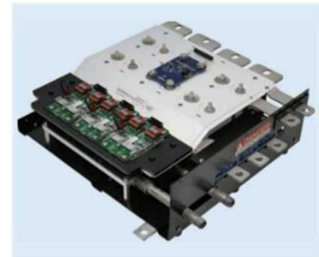
Fig. 13. A compact 16 kg, 250 kW SiC-based three-phase inverter by Wolfspeed [34].
