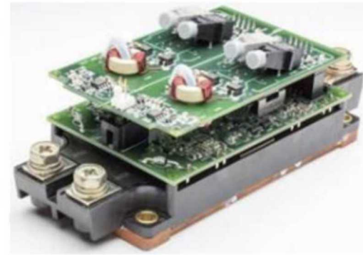
Fig. 14. A 1.7 kV/480 A SiC module with gate driver developed by General Electric [143].
