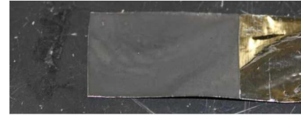
DW \text{LiFePO}_4 on copper current collector
