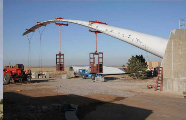
45 m blade test NREL/NWTC, CO
