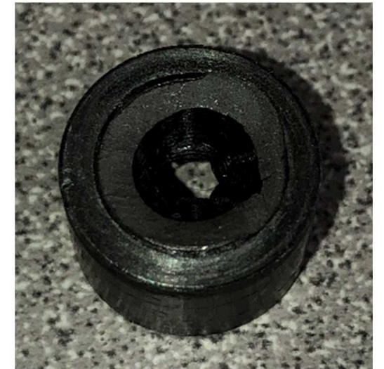
Bottom view: fractured defective socket head bolt
