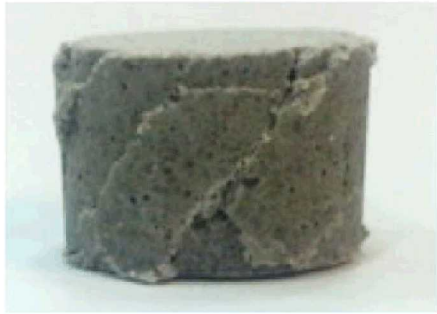
Figure 7. Shear cracks formed during plateau region on syntactic foam. Ahmadi et al., 2014
