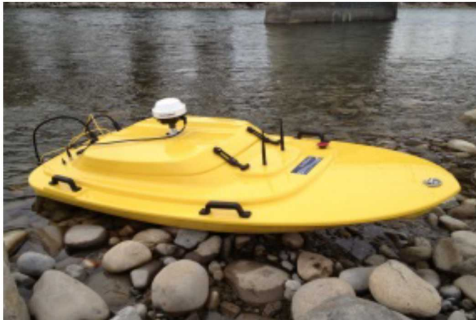
Remote control boat with RTK GPS
