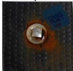
Corrosion of Metal - Carbon Fiber Composite
