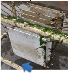
Biofouling & Environmental Effects on Composites
