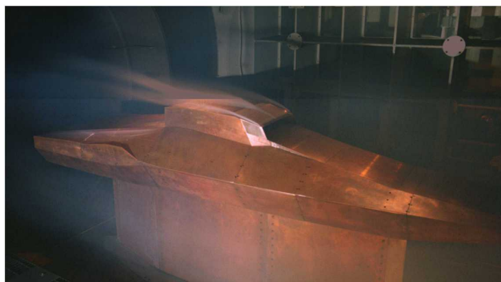
NASA X-43A experimental unmanned hypersonic vehicle (left) CFD simulation of Mach 7 flight (right) Mach 7 wind tunnel test full-scale X-43A. Images courtesy of www.dfrc.nasa.gov/Gallery/Photo/X-43A/Large/
