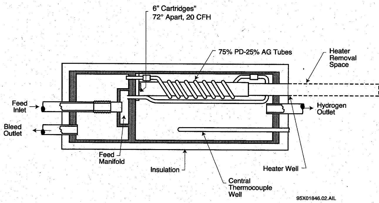
Figure 2. Single Stage RSI Diffuser
