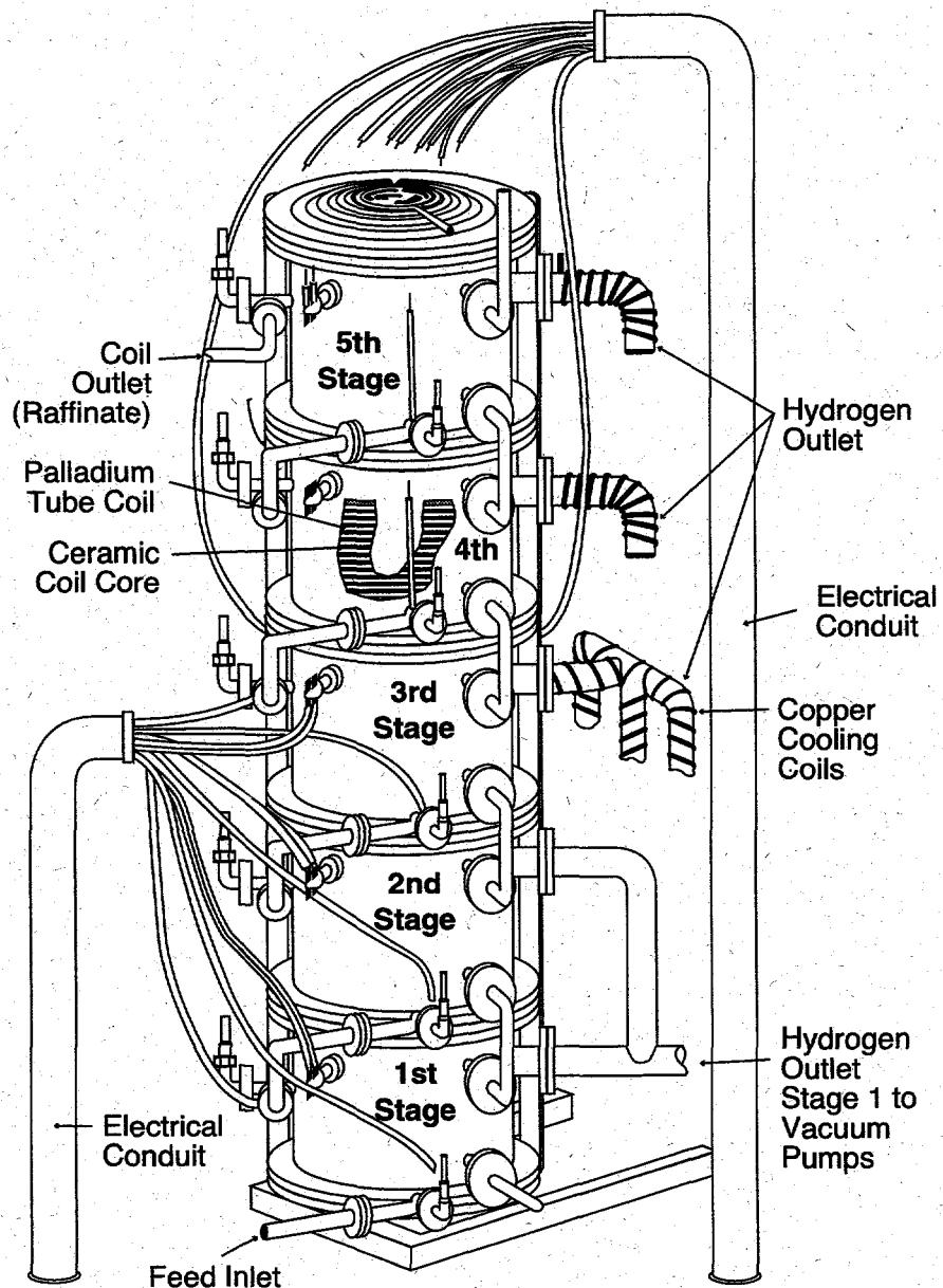
Figure 1. Multistage Palladium Diffuser
