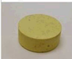
50 wt% AgI/50 wt% Glass 500°C for 3 hr
