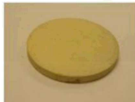
50 wt% AgI/50 wt% Glass, 500°C for 3 hr
