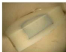
Glass shell, AgI/glass core, 75/25
