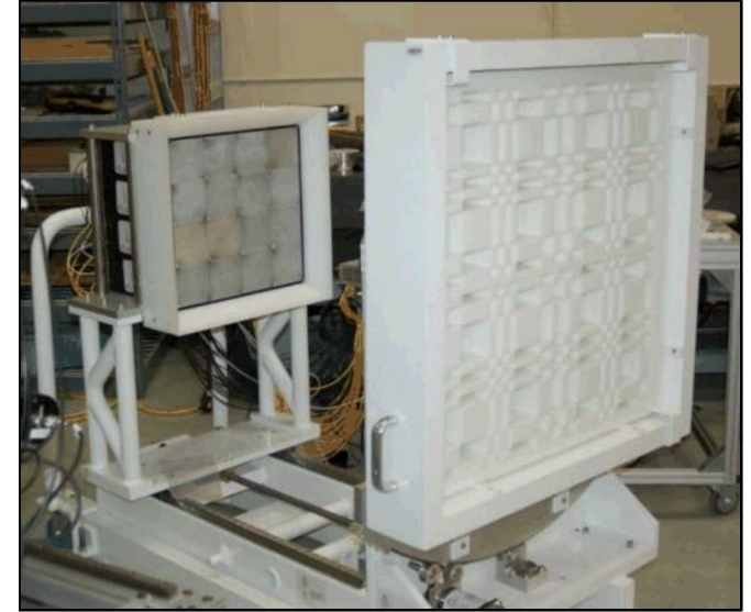
APNIS scanner 32 detectors 3200 pixels
