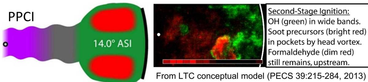
Some R&D: Fuel property and mixture preparation effects on ignition and combustion rate; in-cylinder CO & UHC mitigation
