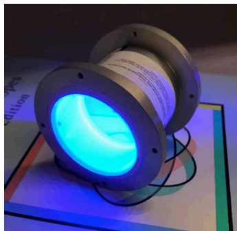
EJ-309: PSD- capable organic liquid scintillator
