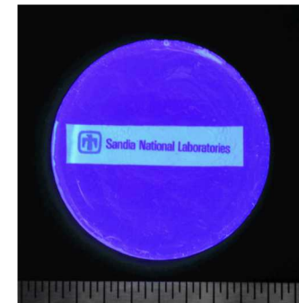
Organic Glass: PSD- capable organic glass scintillator
