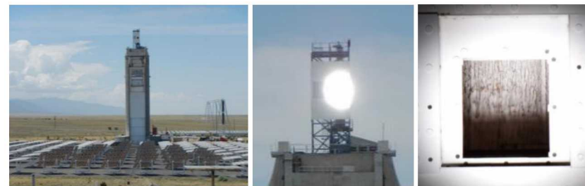
On-sun testing of the falling particle receiver at Sandia National Laboratories
