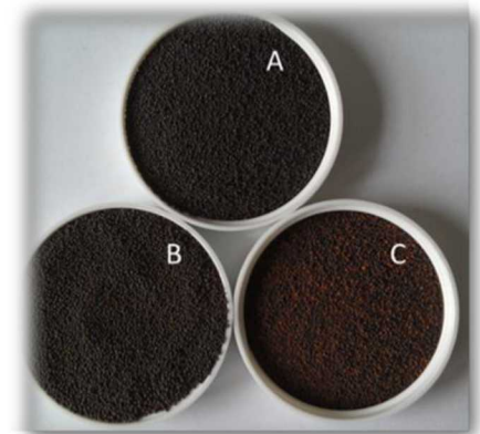
CARBO ceramic particles ("proppants")
