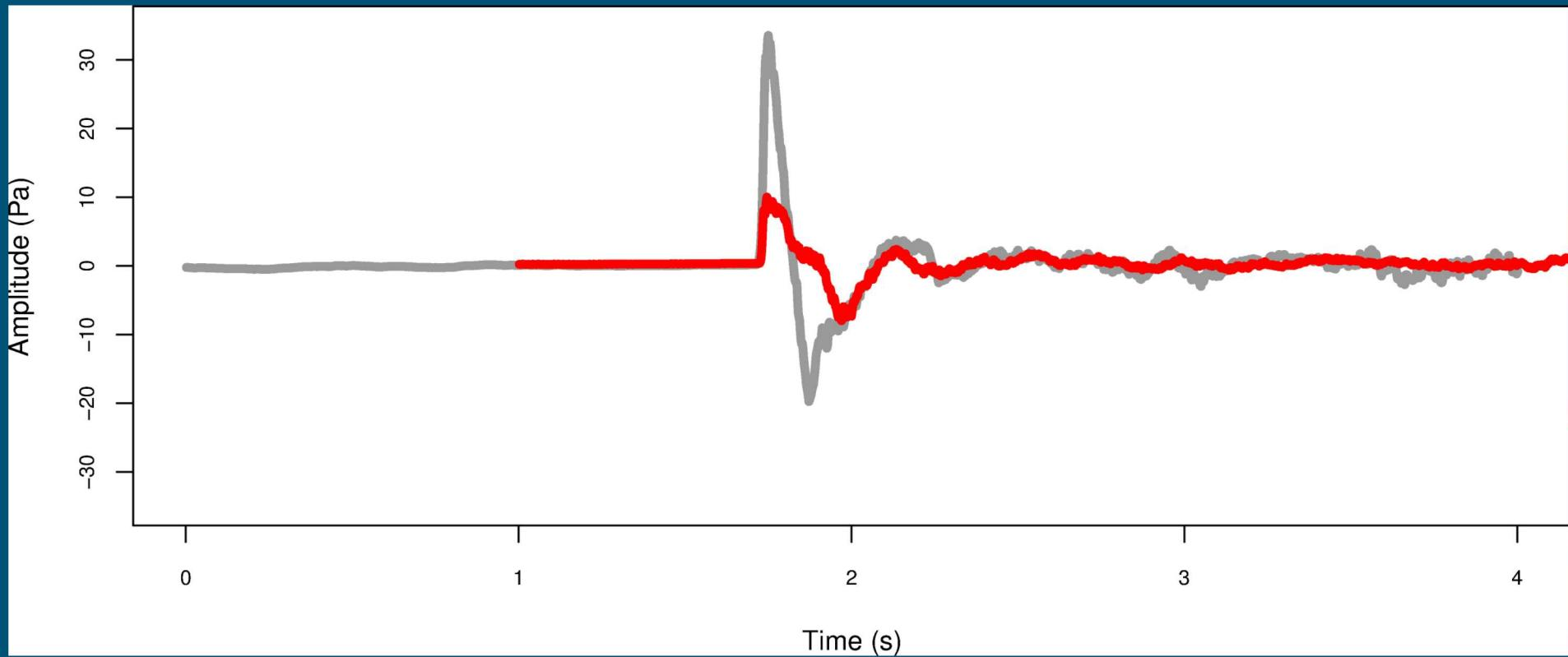
Two identical co-located explosions (800 kg TNT equivalent yield) detonated 90 minutes apart recorded on the same sensor.
