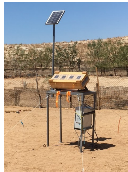
Fig 5: Lab-scale EDS film test setup in Chile
