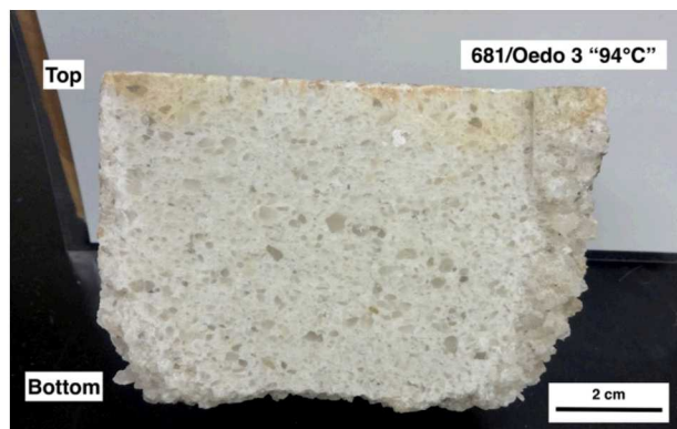
Figure 1: Oedometer test samples as received from IfG, prior to preparation of thick-thin sections.
