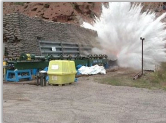
Large bore powder gun – measures differences in performance of weapon materials of interest.
