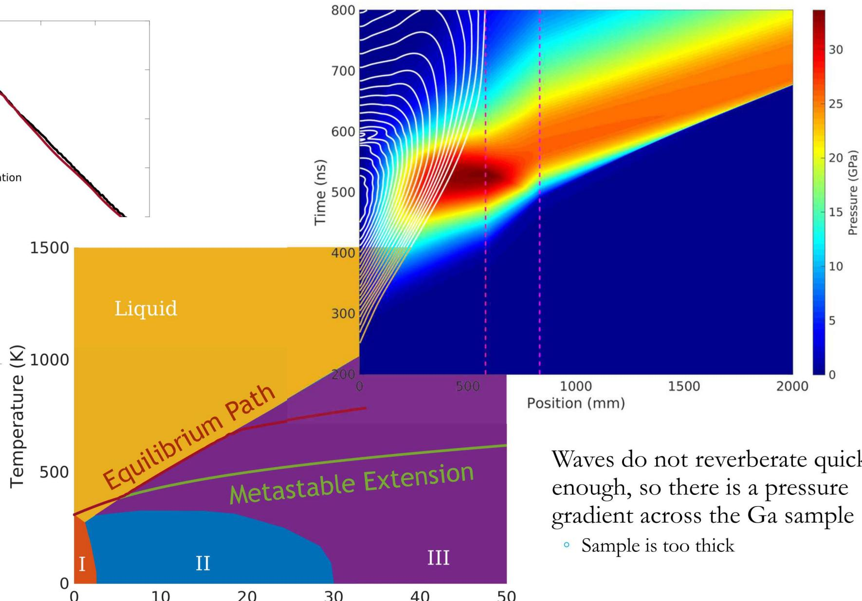
Waves do not reverberate quickly enough, so there is a pressure gradient across the Ga sample
