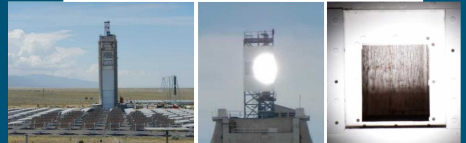
On-sun testing of the falling particle receiver at Sandia National Laboratories
