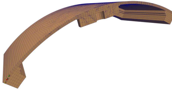
Fig. 3 Cross-section of composite panel in Finite Element Model, showing number of elements in thickness.
