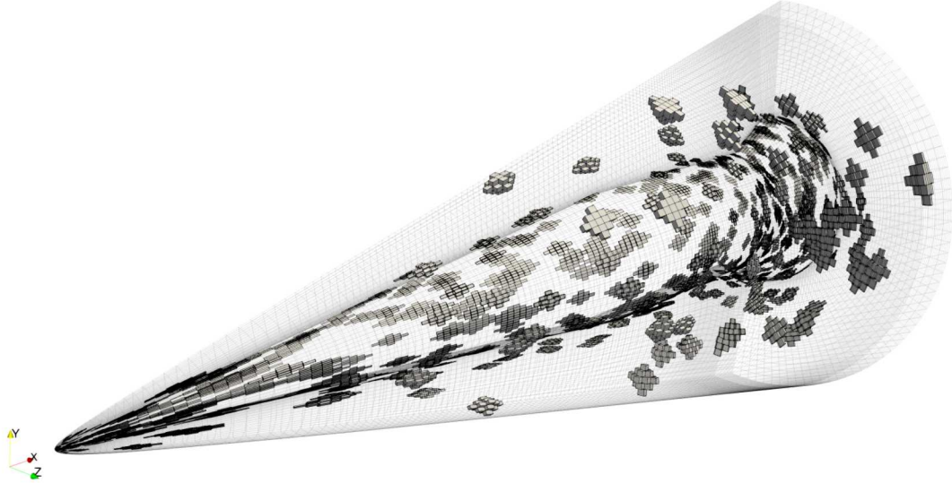
(b) Sample mesh B. The residual is sampled at 813 randomly selected cells (0.04% of all cells), requiring 19901 total cells (0.98% of all cells) to keep neighbors and neighbors of neighbors.
