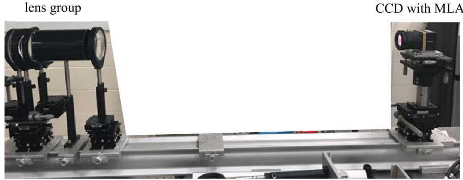
Fig. 1. The custom, high-magnification, long-working-distance plenoptic system.
