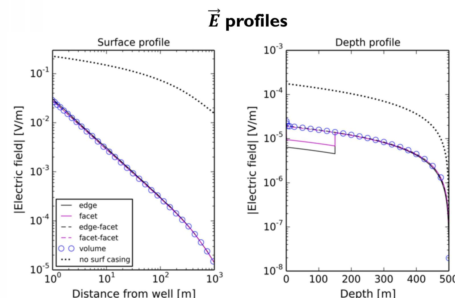
The electric responses are compared against the solution obtained from the fully-volumetric discretization as well as the solution of a single well. The plots indicate that the response of the concentric wells is quite different from the response of a single well. Moreover, the facet-facet and the edge-facet models where the geometry of the outer casing is explicitly defined provide the most consistent results with the fully-volumetric solution.
