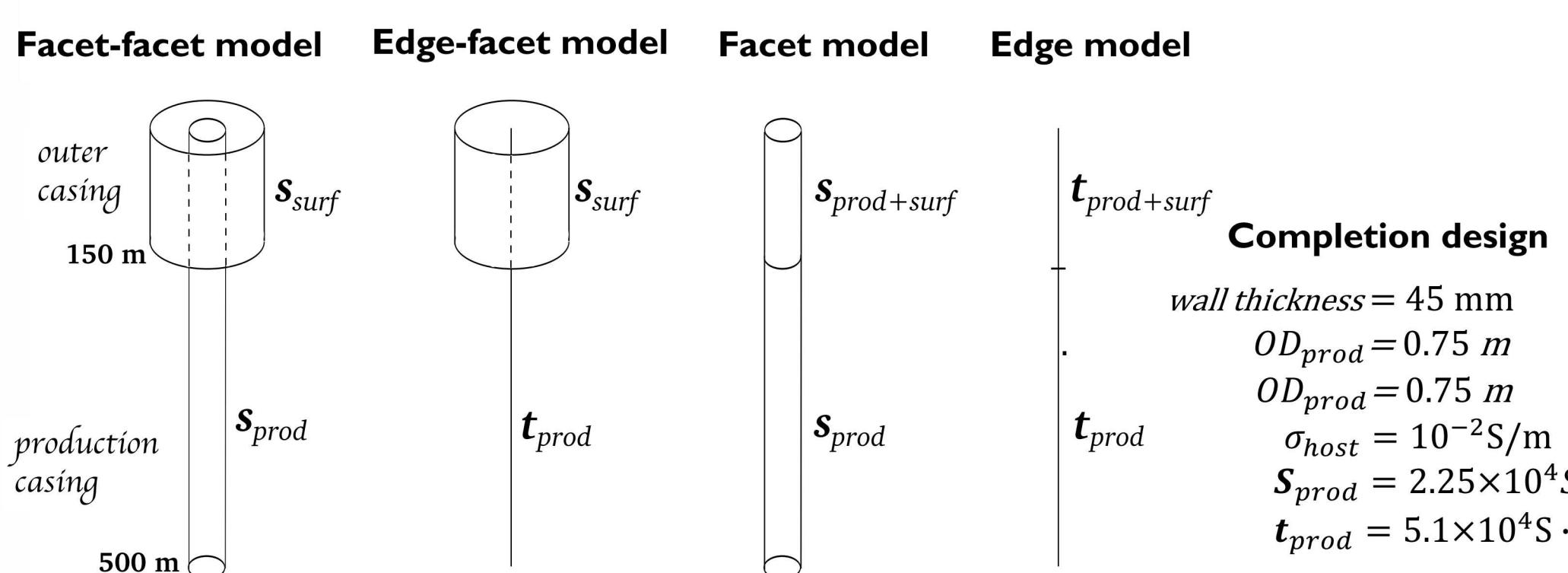
We compare the electric responses obtained from four possible representations of the well completion design to evaluate the efficiency of these discretization approaches on representing the 3D explicit geometric complexity of the well completion design.
