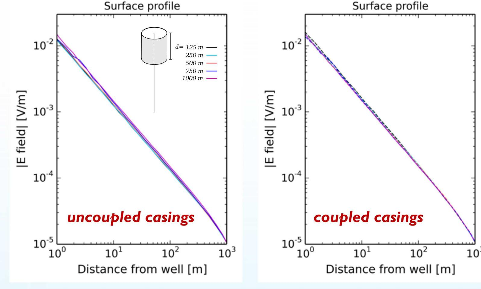
The  $\vec{E}$  surface profiles indicate that the electric response has minor sensitivity to the outer casing length and the coupling between concentric well casings.
