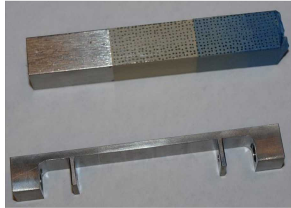
Fig. 5 Applied PSP and speckle pattern on specimen.
