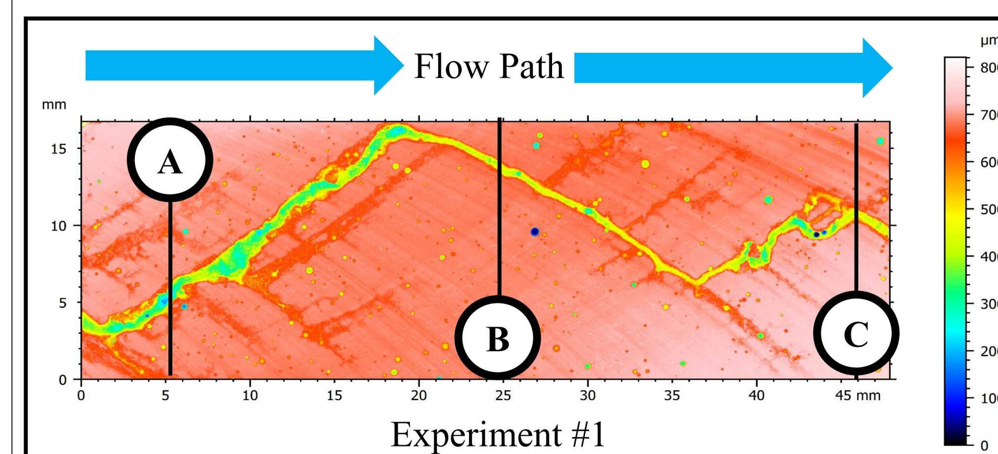
A Nanovea ST400 Profilometer was used to capture the surface roughness of cement before and after being flooded with HCl. The results show a wider deeper channel at the inlet with the channel narrowing and decreasing in depth as the channel migrates further from the inlet. Additionally, the scan shows smaller channel paths, cutting marks, and some pore features.
