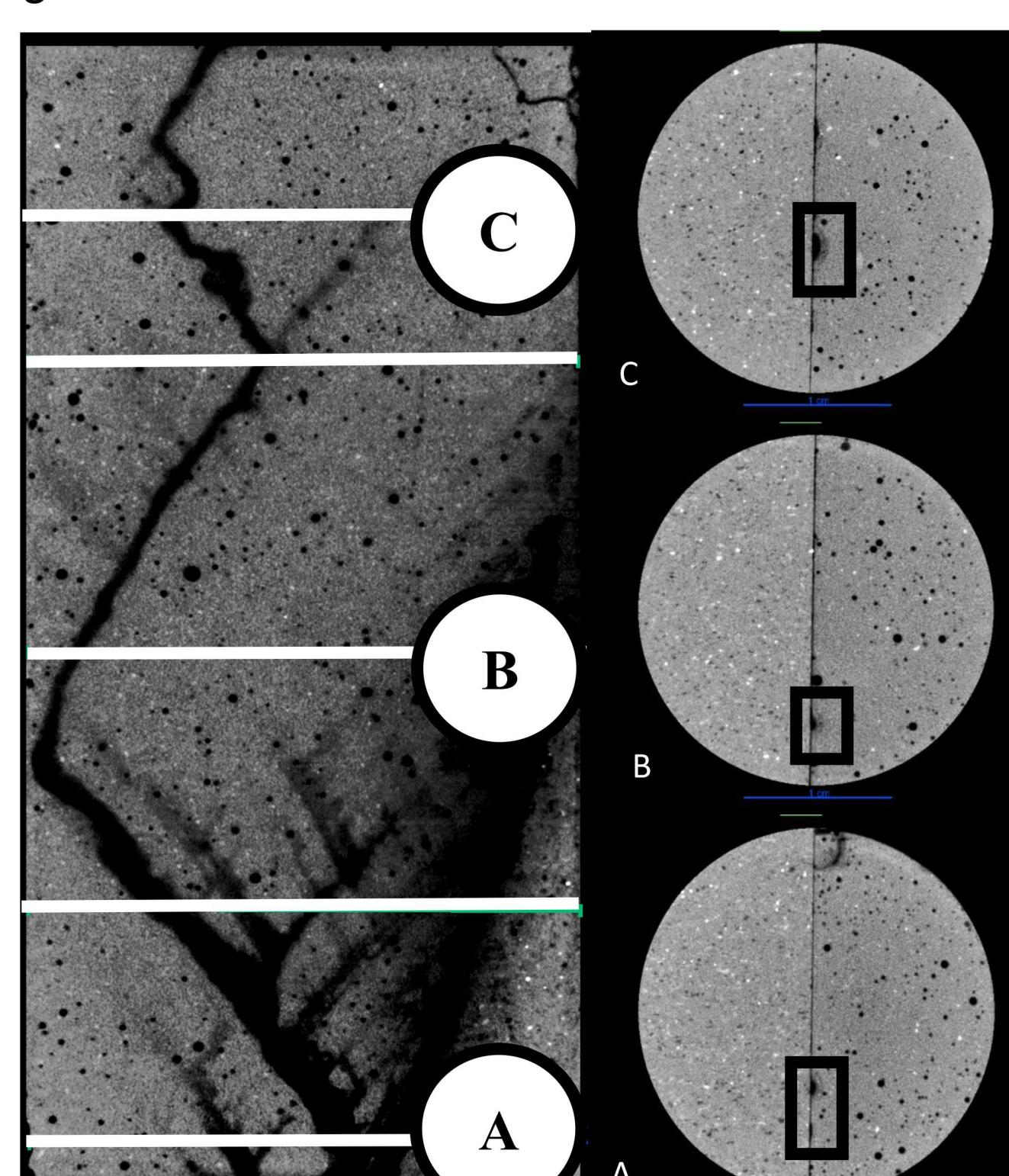
These channel sections will be micro-indented at Vanderbilt University to determine changes in hardness and elastic moduli as a function of distance from the channel.
