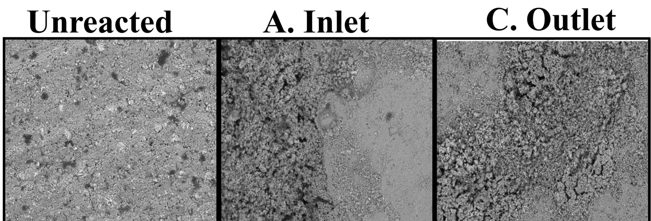
In the presence of water, HCl will self-dissociate into its hydrogen and chlorine atoms. Cement is susceptible to corrosive attacks. At the cement-surface-reservoir interface, hydrogen atoms initiate a reaction propagation front with the calcium hydroxide in the cement. This causes the calcium hydroxide in the cement to dissociate into its calcium and hydroxide atoms. The free calcium then bonds with the free chlorine atoms forming calcium chloride.
