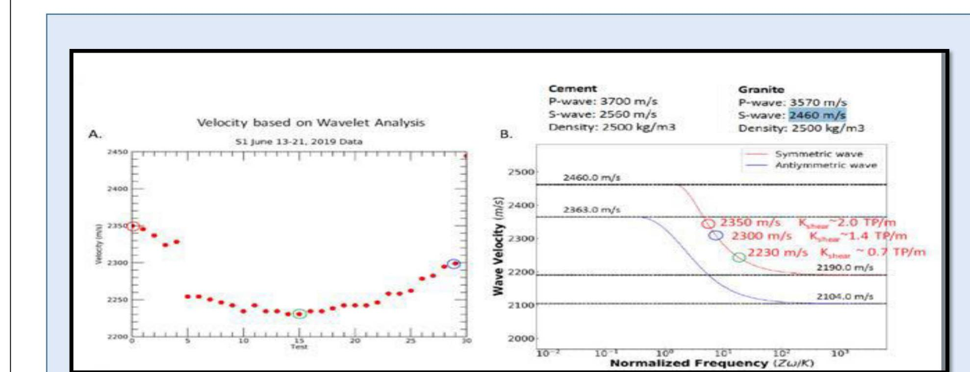
During the course of Test 2, the interface wave velocity is observed to decrease in the first three days of the test, but then shows a slight recovery, possibly due to creep closure. These results suggest that interface waves can detect microannuli degradation.
