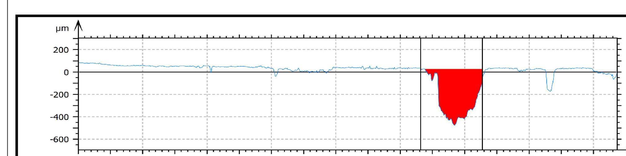
Channel A, pictured above, is 510 μm deep, 555652 μm<sup>2</sup> large, & 2 mm wide. B is 310 μm deep, 156318 μm<sup>2</sup> large, & 1 mm long. C is 313 μm deep, 274709 μm<sup>2</sup> large, & 2.5 mm long.
