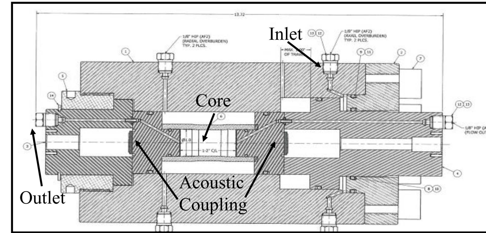
A core-holder with ultrasonic transducers was used to simulate wellbore conditions by providing a constant confining pressure of 13.3 MPa, an axial load of 16.8 MPa, and a temperature of 65°C. All data was recorded and saved in a data logger. A syringe pump flowed pH 3.1 HCl acid through the cement-granite fracture at 4 mL/min. The pH of the effluent solution was recorded with an inline pH probe. P & S waves were recorded throughout experiment.
