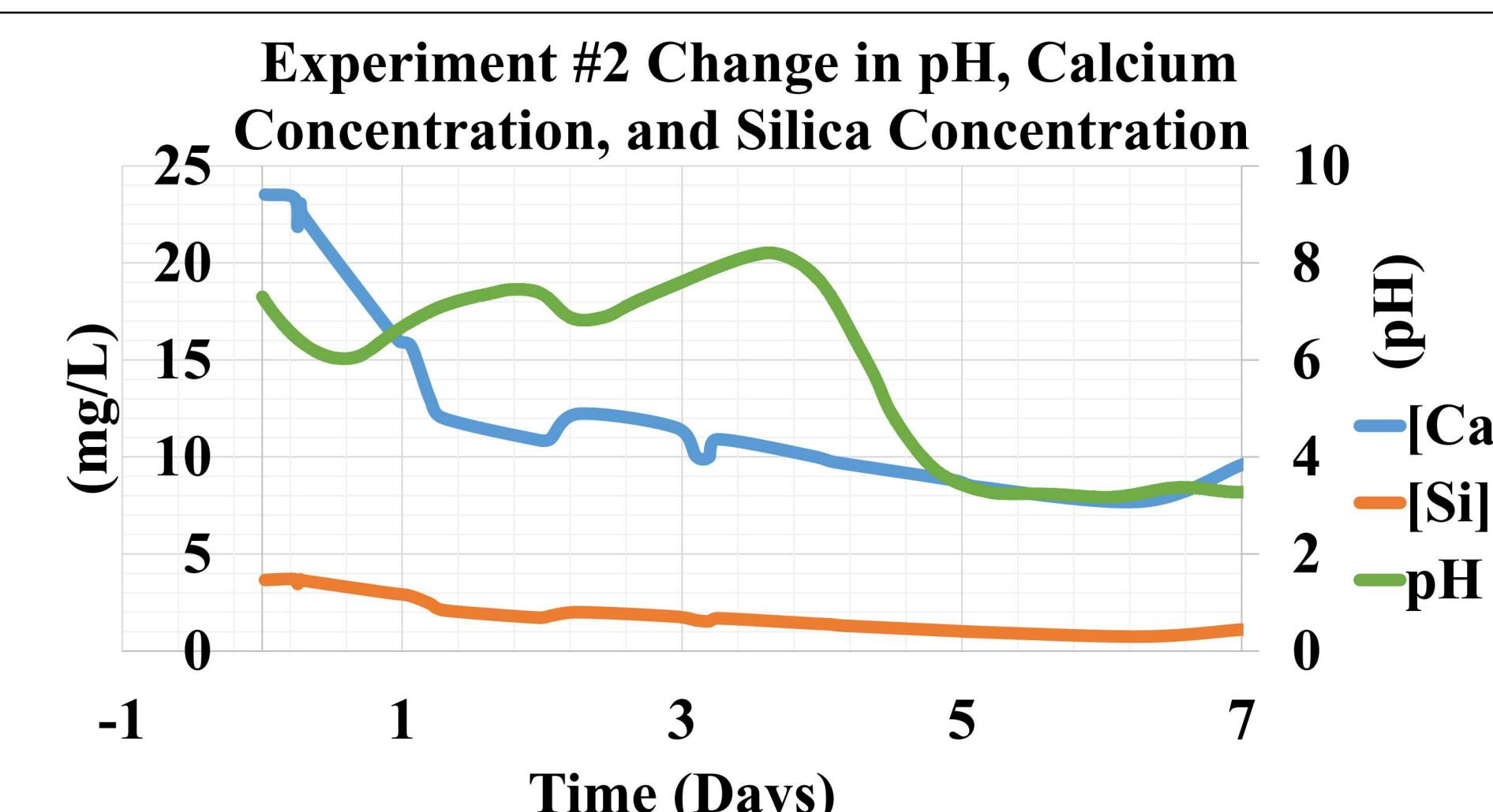
The initial surface reaction between the HCl and cement caused the pH and the [Ca] to rise. Eventually, the reaction became diffusion controlled causing the dissolution rate to decrease.
