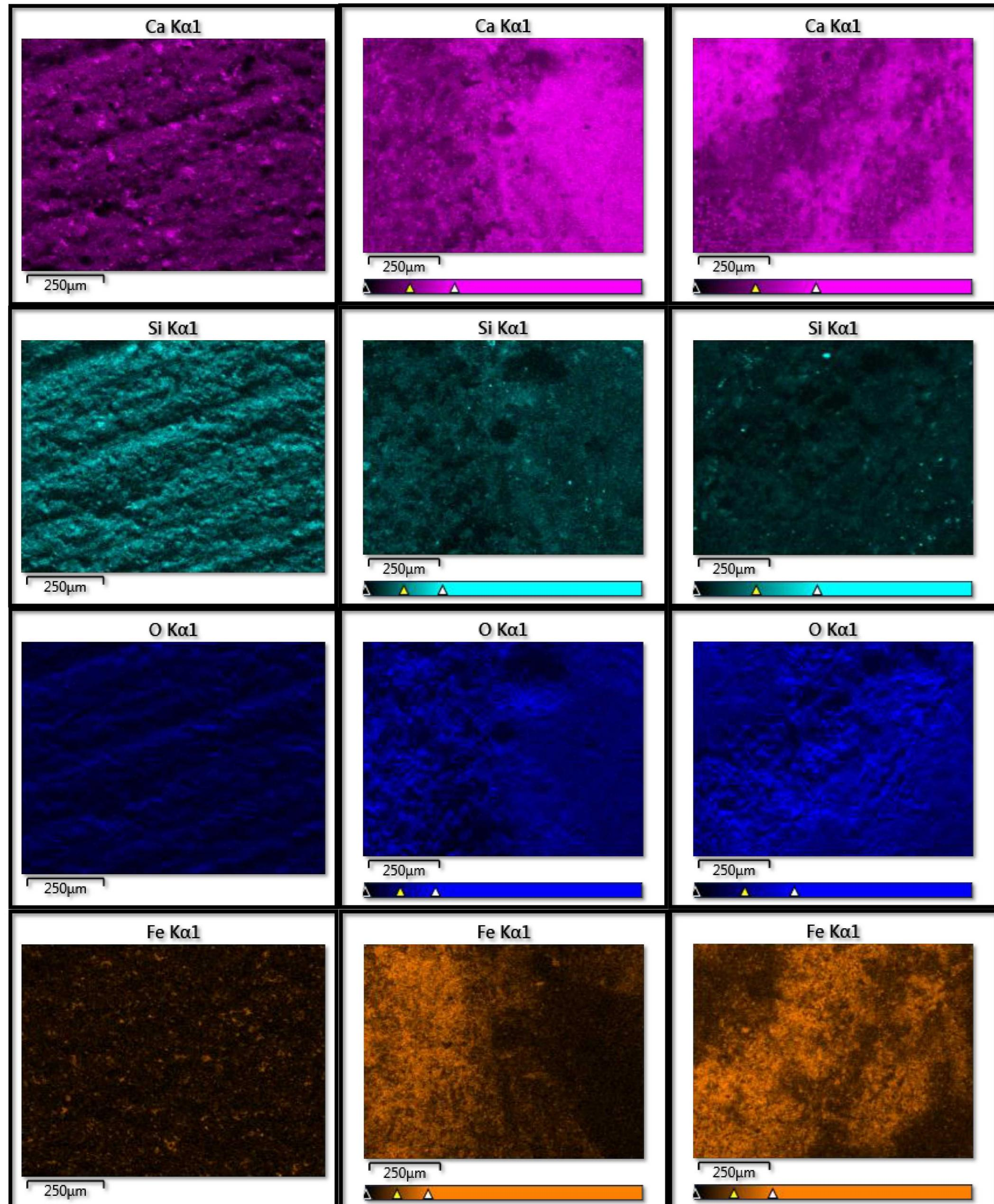
The results show a decrease in Ca and Si in the channels with an increase of Fe and O in the channels. The Fe and O are likely responsible for the orange coloring left behind in the channel's flow path.
