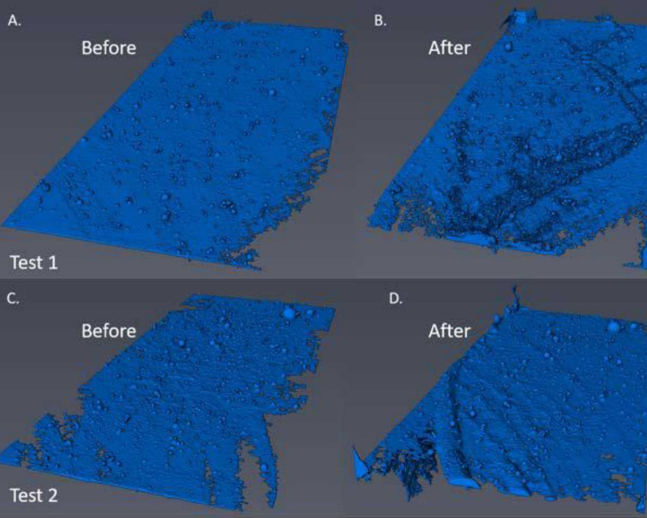
CT scanning was performed before and after each flow through experiment. Reconstruction involves meshing for CFD and other modelling efforts.
