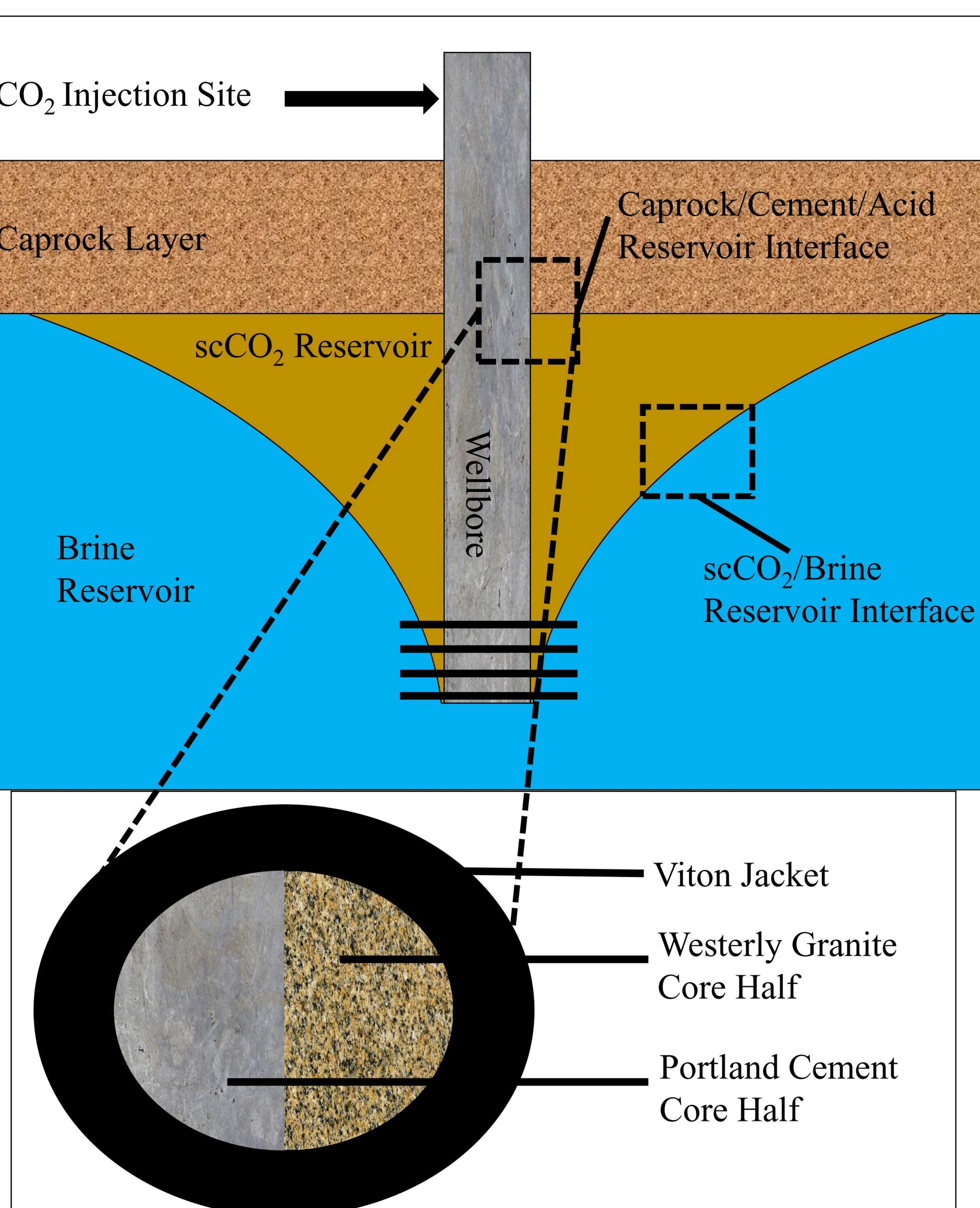
A two inch in length and one inch in diameter core made half of Type G cement and half of granite was fabricated to make a representative sample of the caprock/cement interface. The sample was wrapped in Teflon and then loaded into a Viton jacket, which was then inserted into a pressure vessel for fluid flow and acoustic testing.
