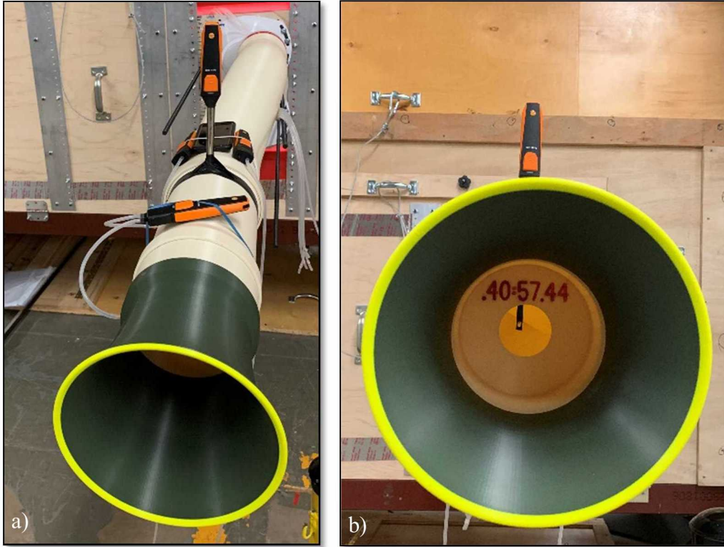
Fig. 4 a) Duct inlet outside the wind tunnel with choke section and b) close-up view down the inlet of the choke and hot wire anemometer.
