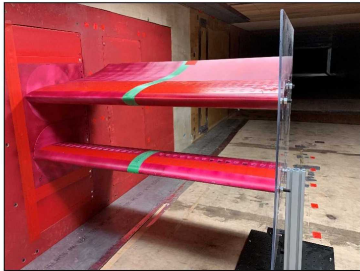
Fig. 3 A 0.5 m chord AeroMINE pair mounted in the wind tunnel. The green ribs contain static pressure taps along the low-pressure side of the foils.
