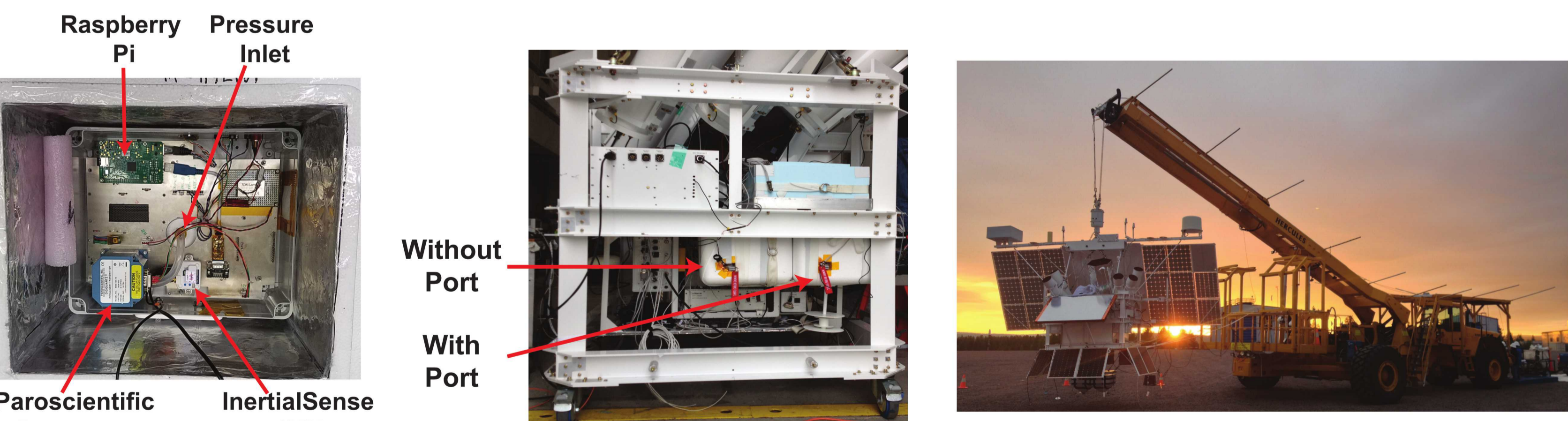
Figure 2: (Left) Assembly of the PIMA payload (Middle) PIMA-1 and 2 integrated on the gondola (foreground, with the red tags) (Right) PMC-Turbo gondola prior to launch (Middle and right images courtesy of Christopher Geach, UMN)
