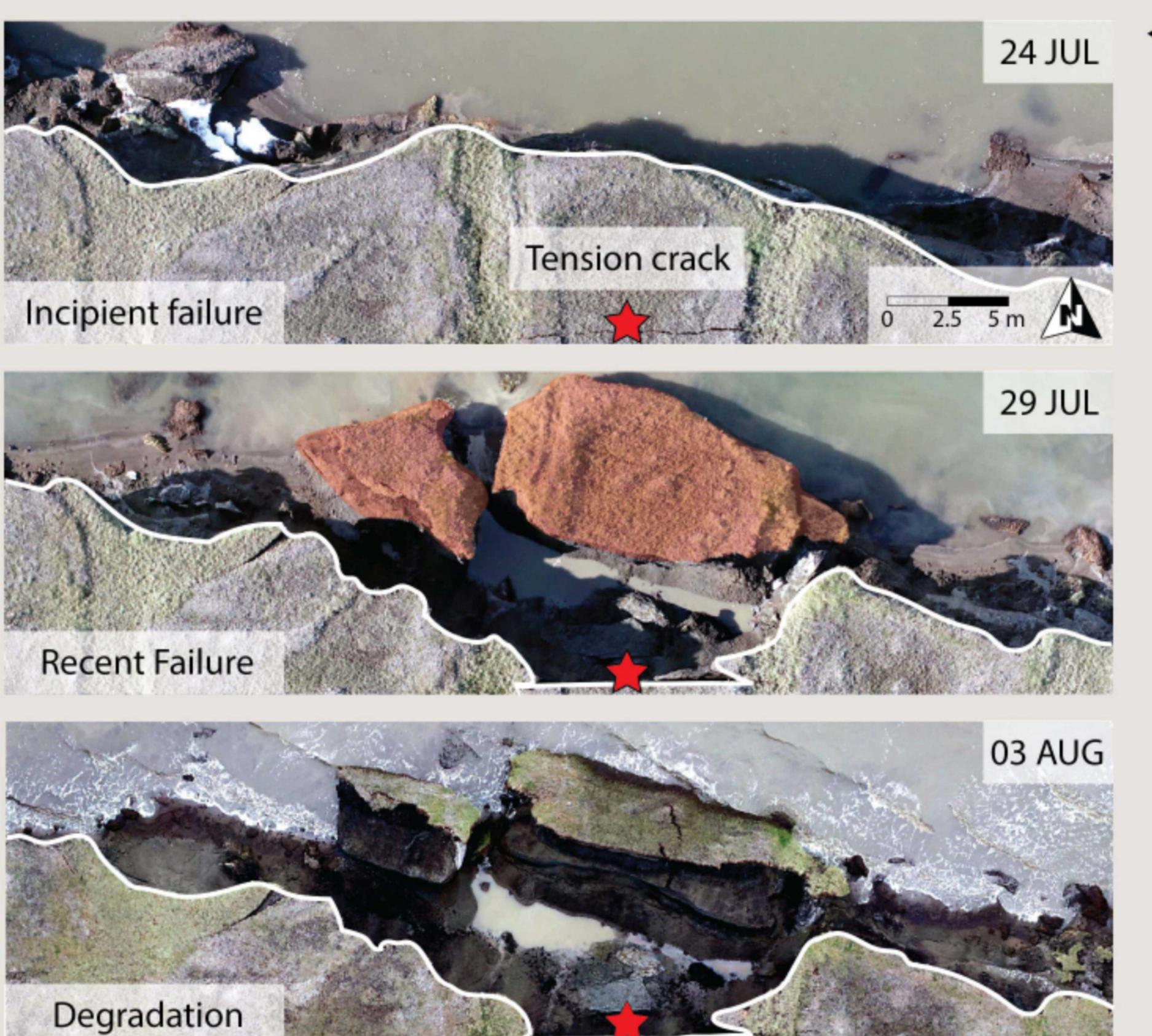
Storms raise nearshore water levels and undercut the bluffs via thermo-abrasion until a toppling mode bluff failure occurs.
