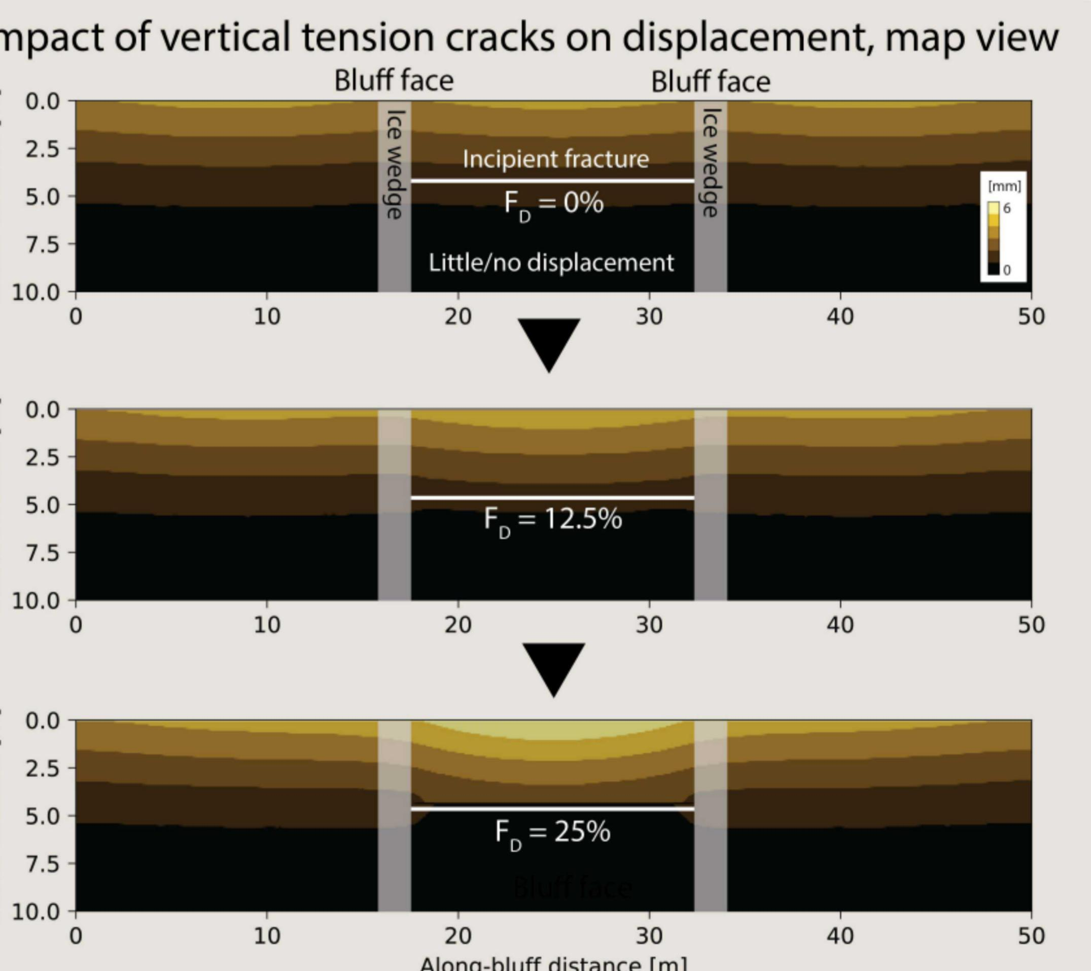
As fracture depth ( $F_D$ ) increases, the displacement field transitions from a relatively uniform (along-bluff) pattern to a more concentrated pattern with the maximum displacement located in the section of the bluff face that is seaward of the map-view fracture midpoint.
